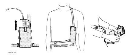
5. To get the Syringe Driver out of the Cover, hold the Cover without squeezing it and press firmly on either end of the Syringe Driver until it pops out.
