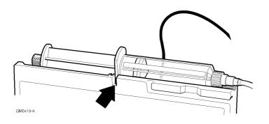
Move the actuator up to the syringe plunger, by pressing and holding in the button on the side, and sliding it along. The push-button on the plunger of the syringe must be fitted in the slot in the actuator. Be careful not to push the plunger forwards.
